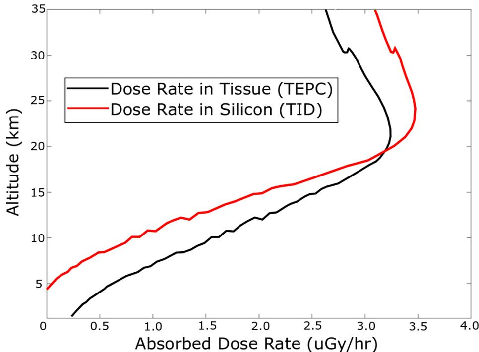
Flight-averaged TID measurements show good agreement to the TEPC measurements
