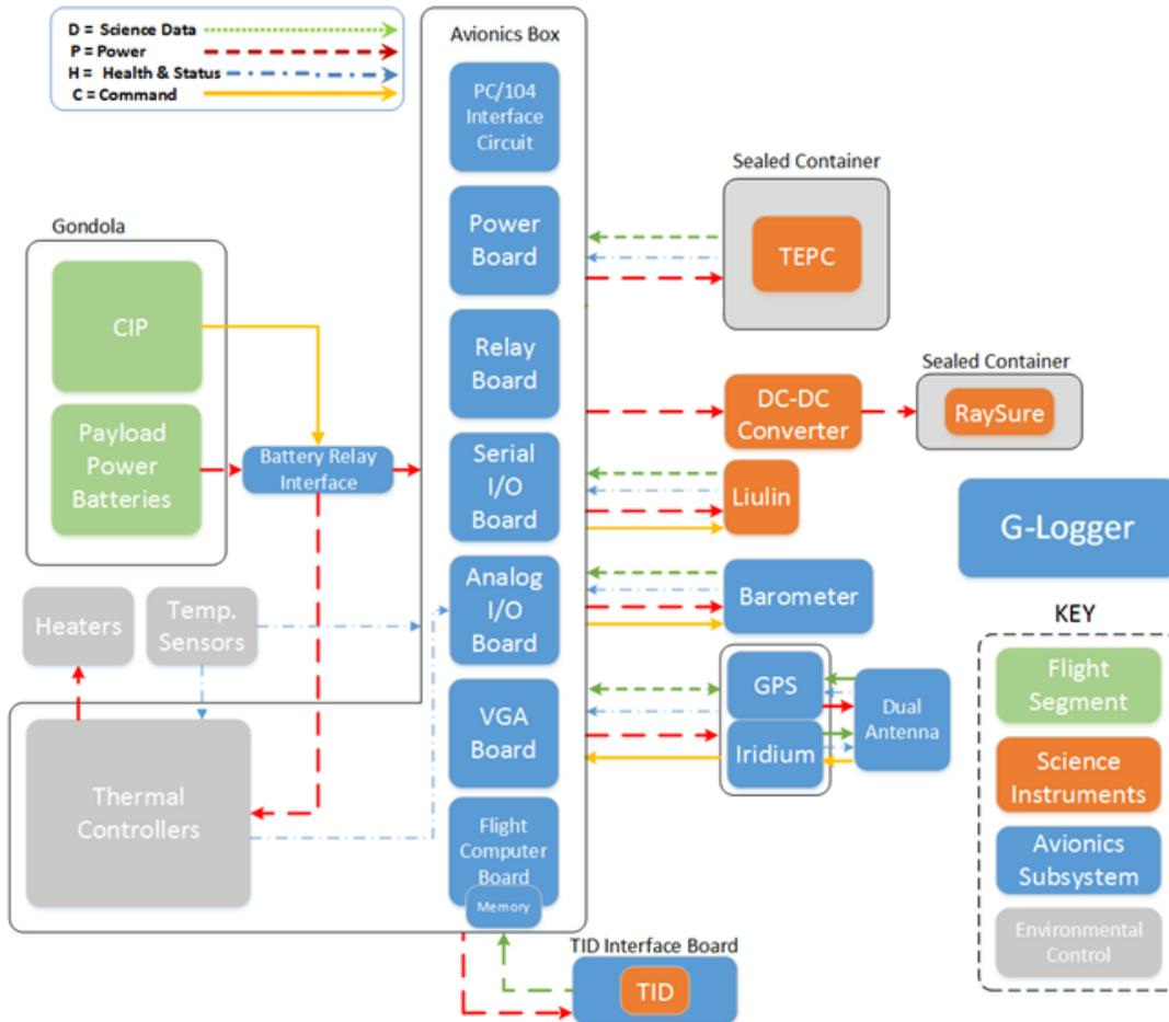
All avionics are COTS with exception of PC/104 Interface Circuit, TID Interface Circuit, and most cables
