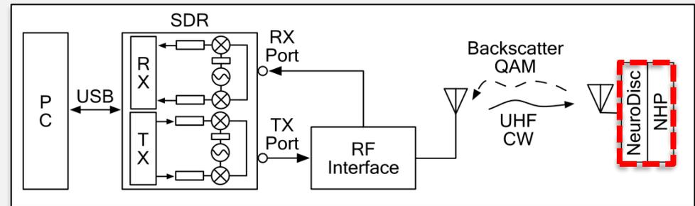
Experimental setup: Receiver had direct line-of-sight at 0.3 m. Uplink rate was 6.25 Mbps.
