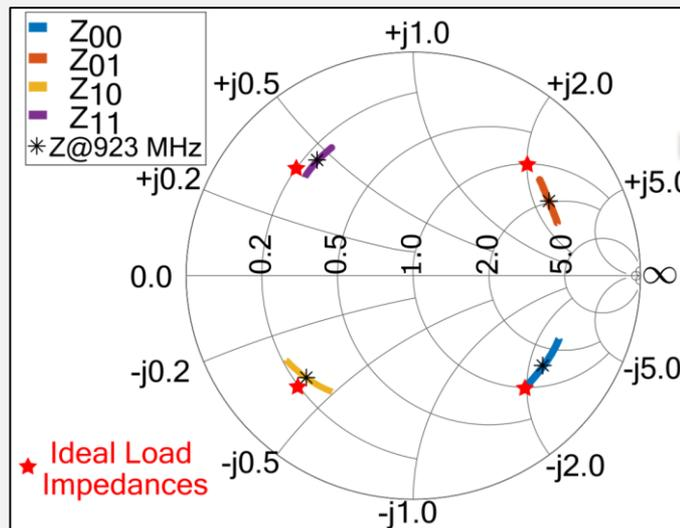
**Measurement of the RF switch states
