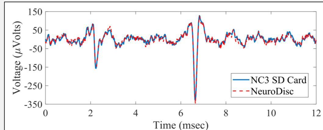
**Comparison of the same pre-recorded data wirelessly uplinked by the NeuroDisc and saved on the NC3 SD card**
