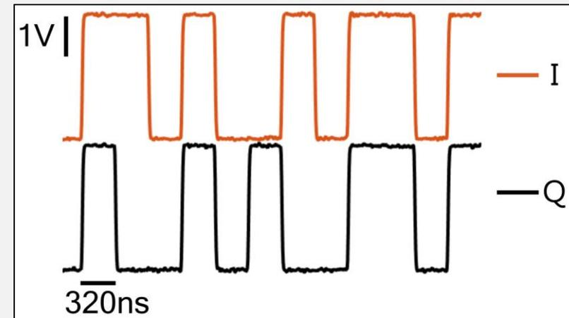
**DQPSK state machine encodes the data into modulator control signals**
