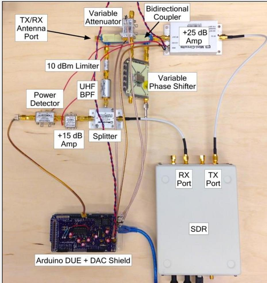
Open-source software-defined radio system with self-jammer cancellation
