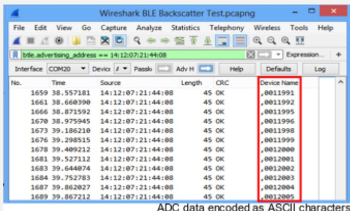
**Analog sensor data is uplinked in BLE-compatible advertising packets to any unmodified BLE receiver**
