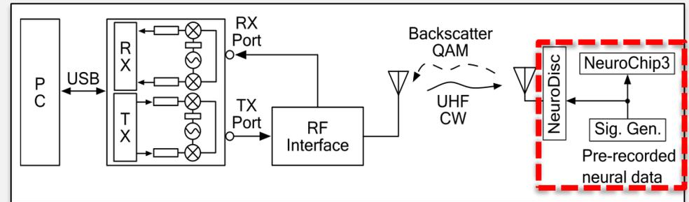
**Experimental setup: Receiver had direct line-of-sight at 0.3 m.
