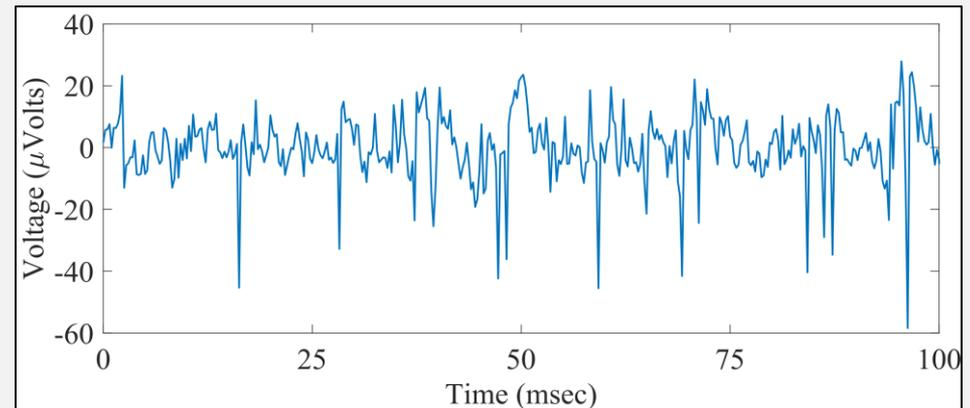
One of eight channels measured at 5 kHz with BPF between 1 Hz – 2 kHz
