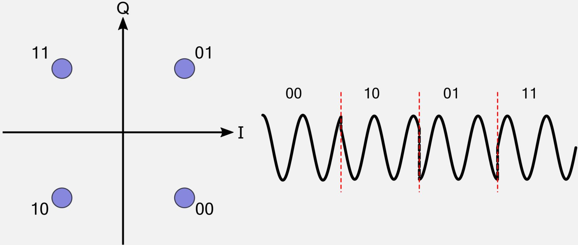
QPSK modulation encodes 2 bits per symbol
