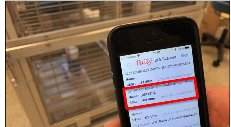
**Successful reception of packets outside the cage on an unmodified smartphone**
