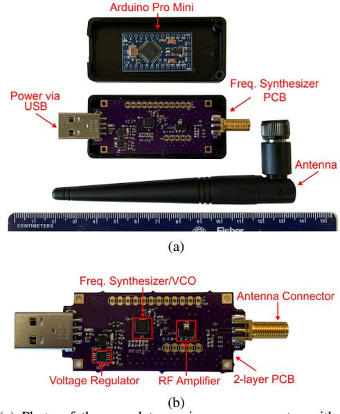
Fig. 3. (a) Photo of the complete carrier wave generator with a 2.4 GHz antenna (b) Zoomed-in photo of the frequency synthesizer printed circuit board (PCB)
