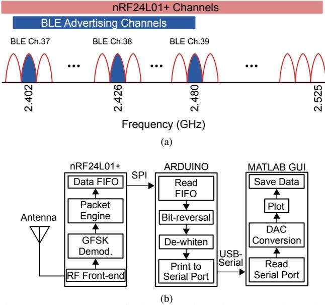
Fig. 2. (a) Frequency range for the nRF24L01+ chip and BLE ISM band (b) Block diagram showing data path of received signal
