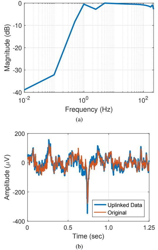
Fig. 5. Plots of (a) the measured frequency response of the wireless BCI and (b) Pre-recorded neural data uplinked to the receiver versus the original data
