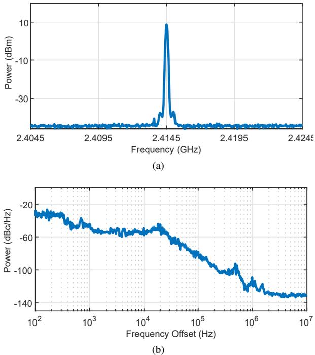
Fig. 4. Laboratory measurements of the CW generator showing its (a) wideband frequency spectrum and (b) phase noise
