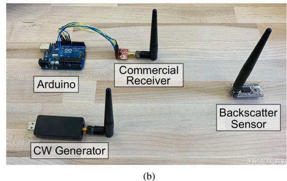
Fig. 1. (a) Cartoon depiction of the presented BCI application with non-human primate subject (b) Photo of receiver, CW generator, and a generic backscatter sensor
