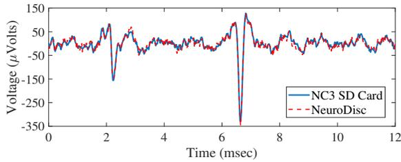
Fig. 5: Plot of pre-recorded neural spike data recorded by the reference BCI (NeuroChip3) and the NeuroDisc. Good agreement can be seen between the two systems.
