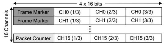
Fig. 3: Packet structure - each packet is 1024 bits long, containing 416 bits of biosignal data prior to ECC
