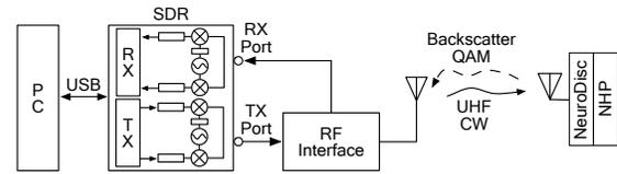
Fig. 6: Test setup for *in vivo* recordings with an NHP.
