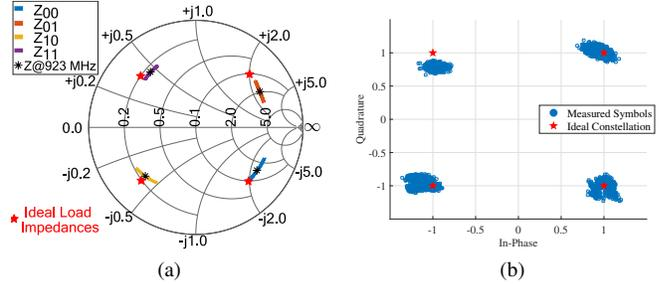
Fig. 4: (a) Impedance measurements of the DQPSK backscatter modulator states across the 900 MHz ISM band (b) Recorded symbol constellation over 5,000 symbol periods with a calculated EVM of 9.69% (adapted from [6])
