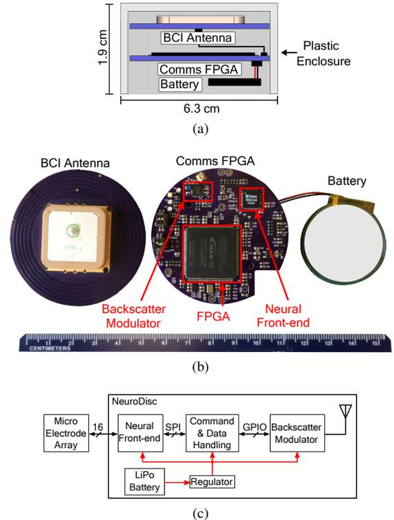
Fig. 1: (a) NeuroDisc mechanical stackup (b) Photo of the NeuroDisc sub-assemblies (c) Block diagram of the Comms FPGA board
