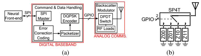
Fig. 2: (a) Comms FPGA data flow detail (b) DQPSK backscatter modulator detail
