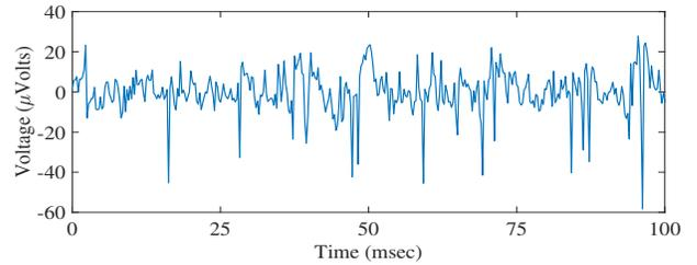
Fig. 7: Example of wirelessly uplinked *in vivo* neural spike recordings from the primary motor cortex of a pigtail macaque.
