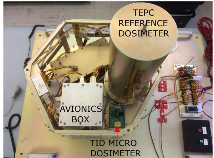
**Fig. 3. Overview photo of the RaD-X payload**
