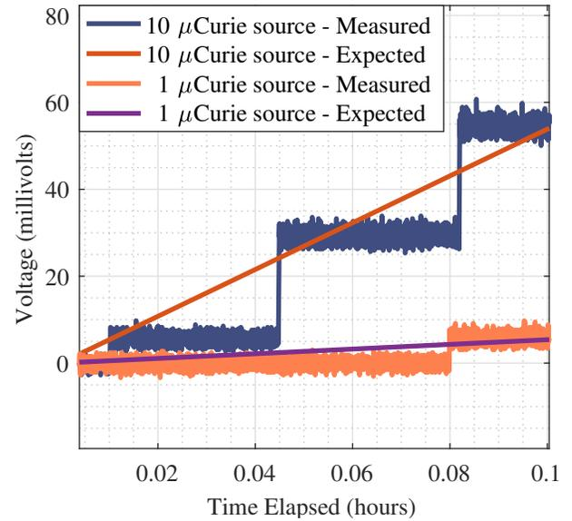
**Fig. 8. Lab measurements versus expected results with Cs-137 source, observed noise  $\sim 7$  mV peak-to-peak**
