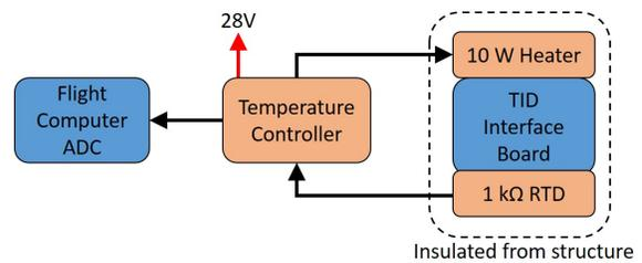
**Fig. 14. Active temperature control system block diagram**
