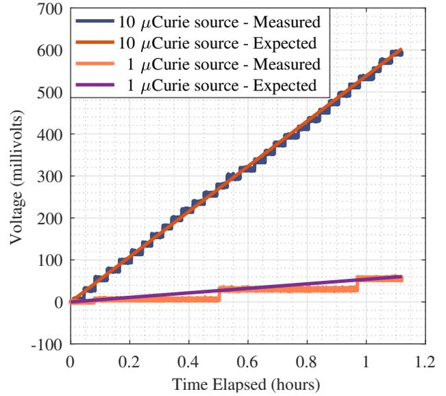
**Fig. 7. Lab measurements versus expected results with Cs-137 source, TID low channel**
