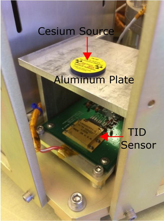
**Fig. 6. Measurement set up with a Cs-137 gamma ray source**
