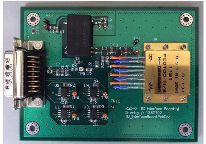
Fig. 5. Photo of the TID interface PCB
