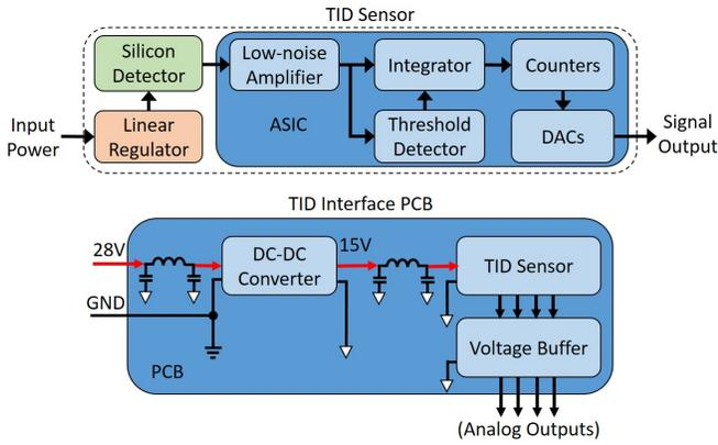
Fig. 4. TID sensor and interface PCB block diagram
