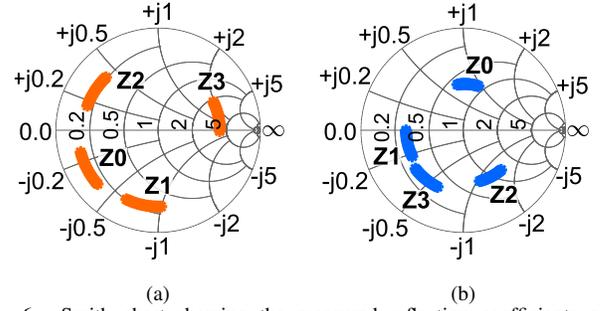
Fig. 6. Smith chart showing the measured reflection coefficients of the backscatter modulator for (a) the 900 MHz ISM band and (b) the 2.4 GHz ISM band.
