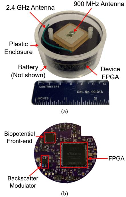
Fig. 2. (a) Photo of the NeuroDisc stack in a plastic enclosure (b) Photo of the NeuroDisc FPGA printed circuit board
