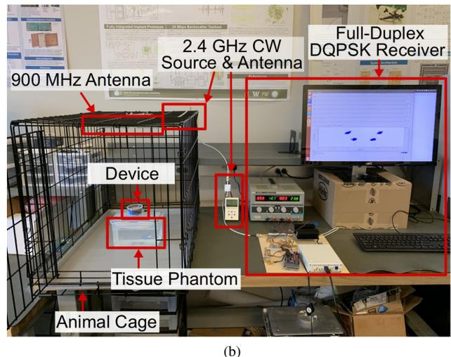
Fig. 1. Example deployment of a wireless neural recorder leveraging a dual-band backscatter data uplink.
