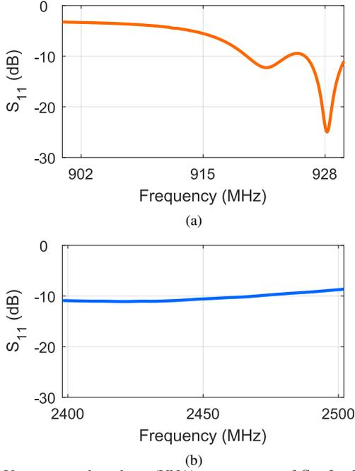
Fig. 5. Vector network analyzer (VNA) measurement of  $S_{11}$  for the dual-band antenna in the (a) 900 MHz ISM band and (b) the 2.4 GHz ISM band.
