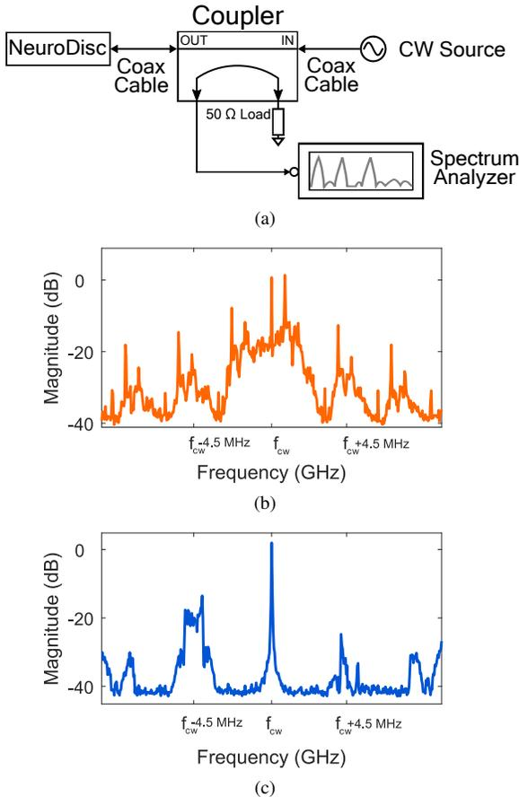
Fig. 7. (a) Block diagram of cabled measurement setup (b) Plot of the measured spectrum for DQPSK packets (c) Plot of the measured spectrum for SSB BLE packets.
