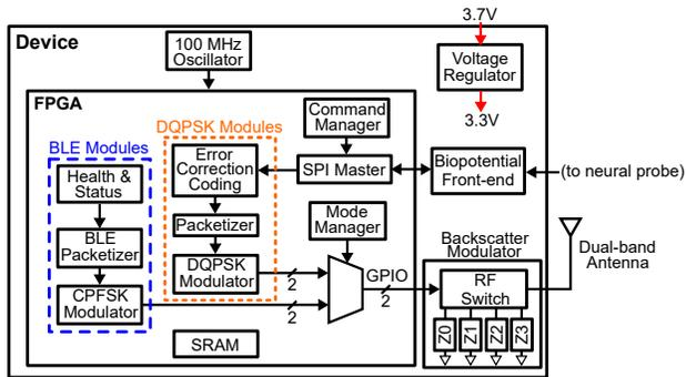
Fig. 3. Block diagram of the FPGA-based digital logic
